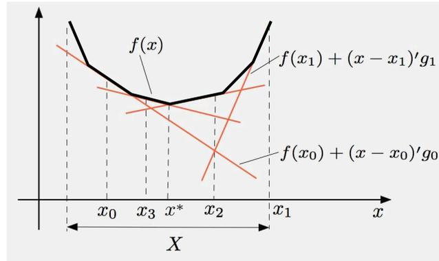
**Figure 6.4.2.** Illustration of the finite convergence property of the cutting plane method in the case where  $f$  is polyhedral. What happens here is that if  $x_k$  is not optimal, a new cutting plane will be added at the corresponding iteration, and there can be only a finite number of cutting planes.
