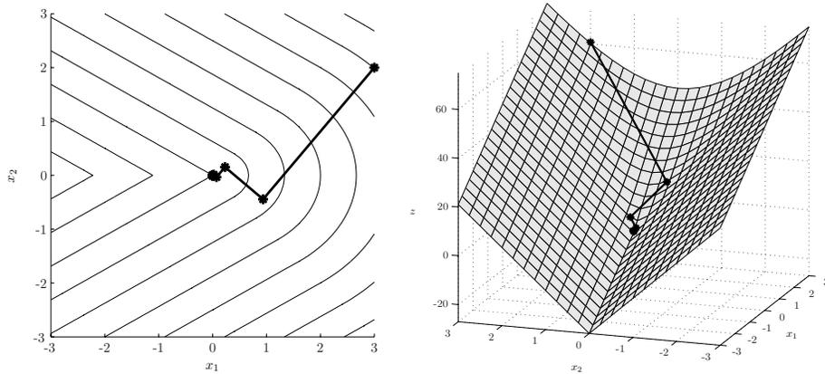
**Figure 6.11.1.** Level sets and steepest descent path for the function of Exercise 6.8. The method converges to the nonoptimal point  $(0, 0)$ .
