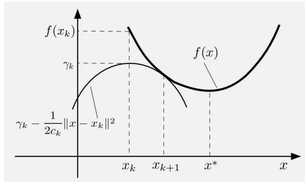
**Figure 6.5.2.** Geometric view of the proximal algorithm (6.145). The minimum of  $f(x) + \frac{1}{2c_k} \|x - x_k\|^2$  is attained at the unique point  $x_{k+1}$  at which the graph of the quadratic function  $-\frac{1}{2c_k} \|x - x_k\|^2$ , raised by the amount
